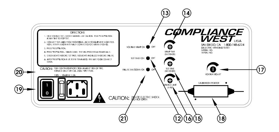
Figure 3-2. Controls, Indicators, Connectors - Model HT-5000 Rear Panel
