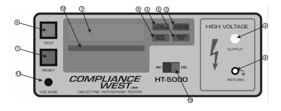
Figure 3-1. Controls, Indicators, Connectors - Model HT-5000 Front Panel
